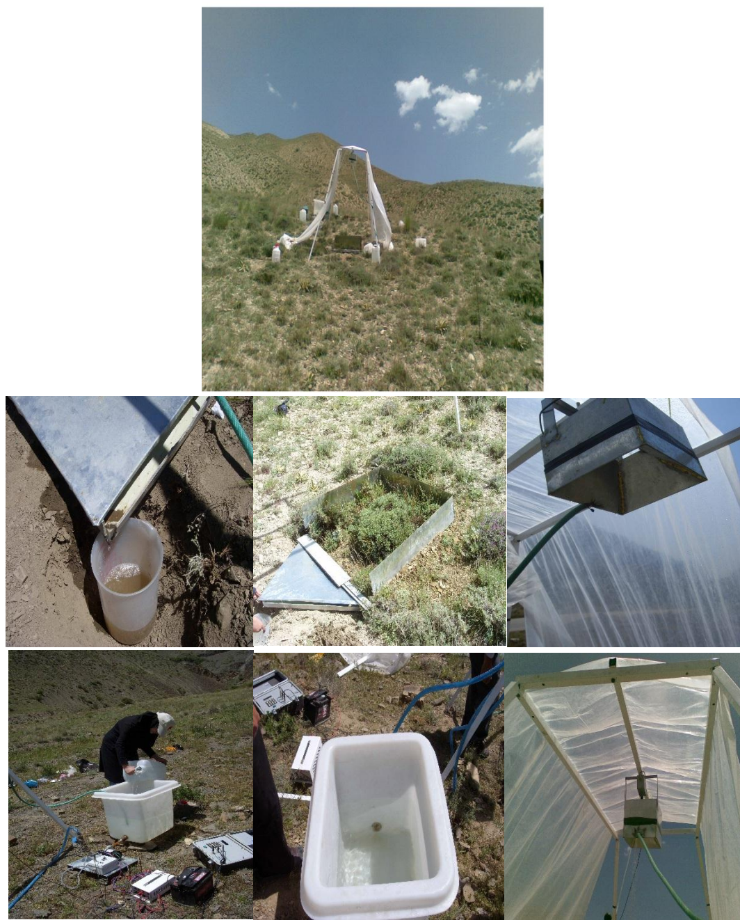
Figure 2 Design and structure of the portable rainfall simulator
