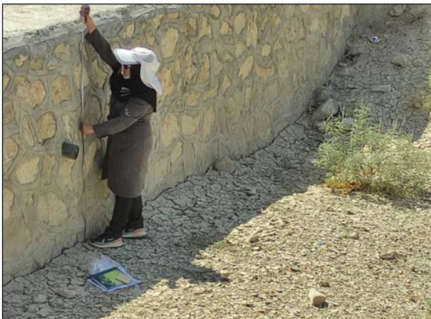
**Figure 3)** Measurement of the sediment deposited depth.
