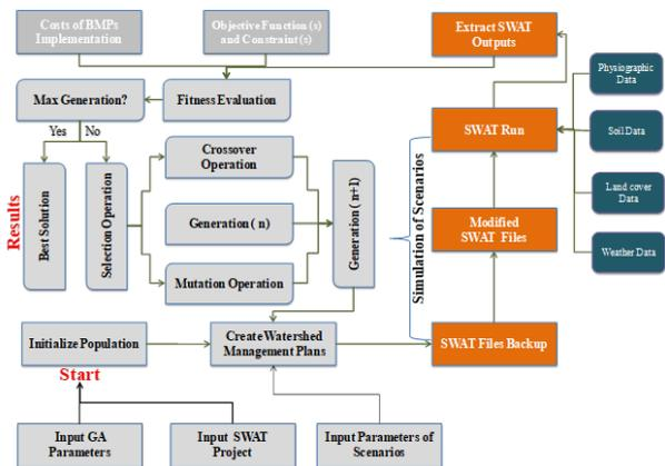
**Figure 1)** Flowchart of the proposed DST in MATLAB computer program including input data, hydrologic model, optimization algorithm, and their interactions
