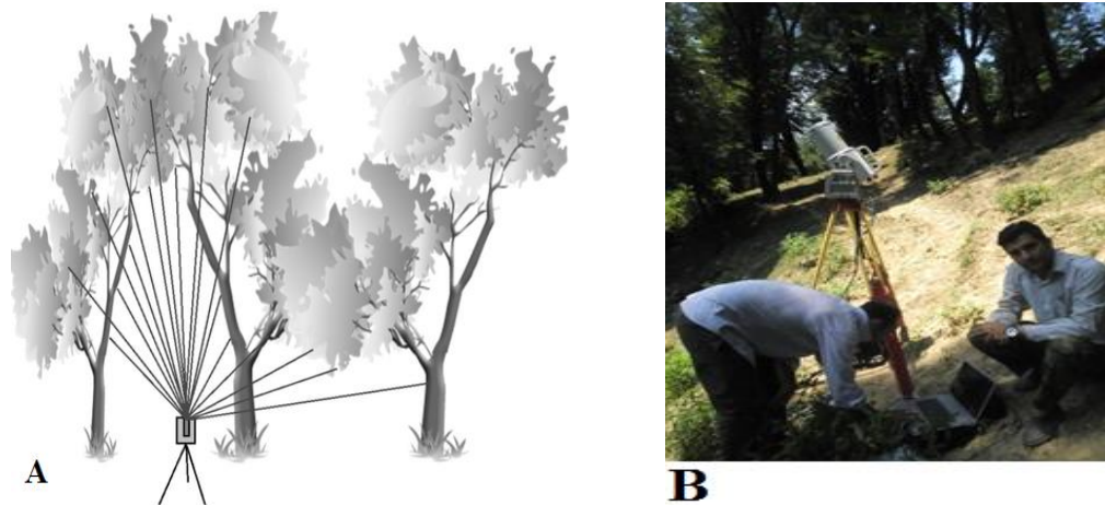
Figure 2 Schematic picture (A) pick up point cloud data by TLS (B) laser scanner field set up
