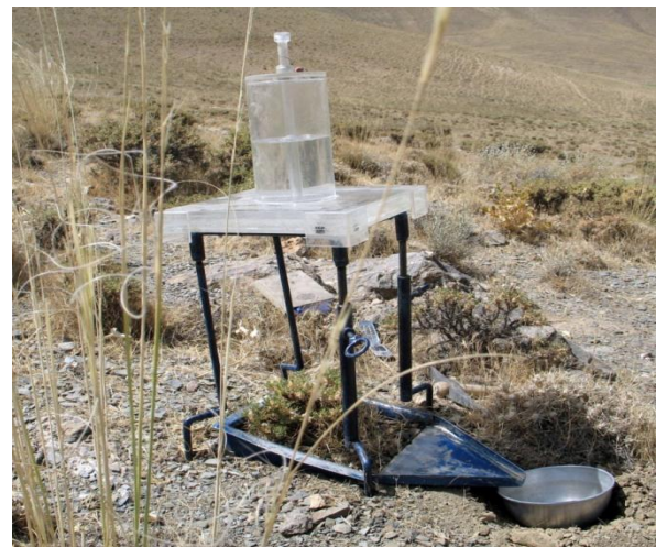
Figure 1 Mounted rainfall simulator in the field
