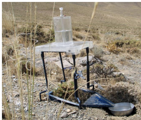
Figure 1 Mounted rainfall simulator in the field
