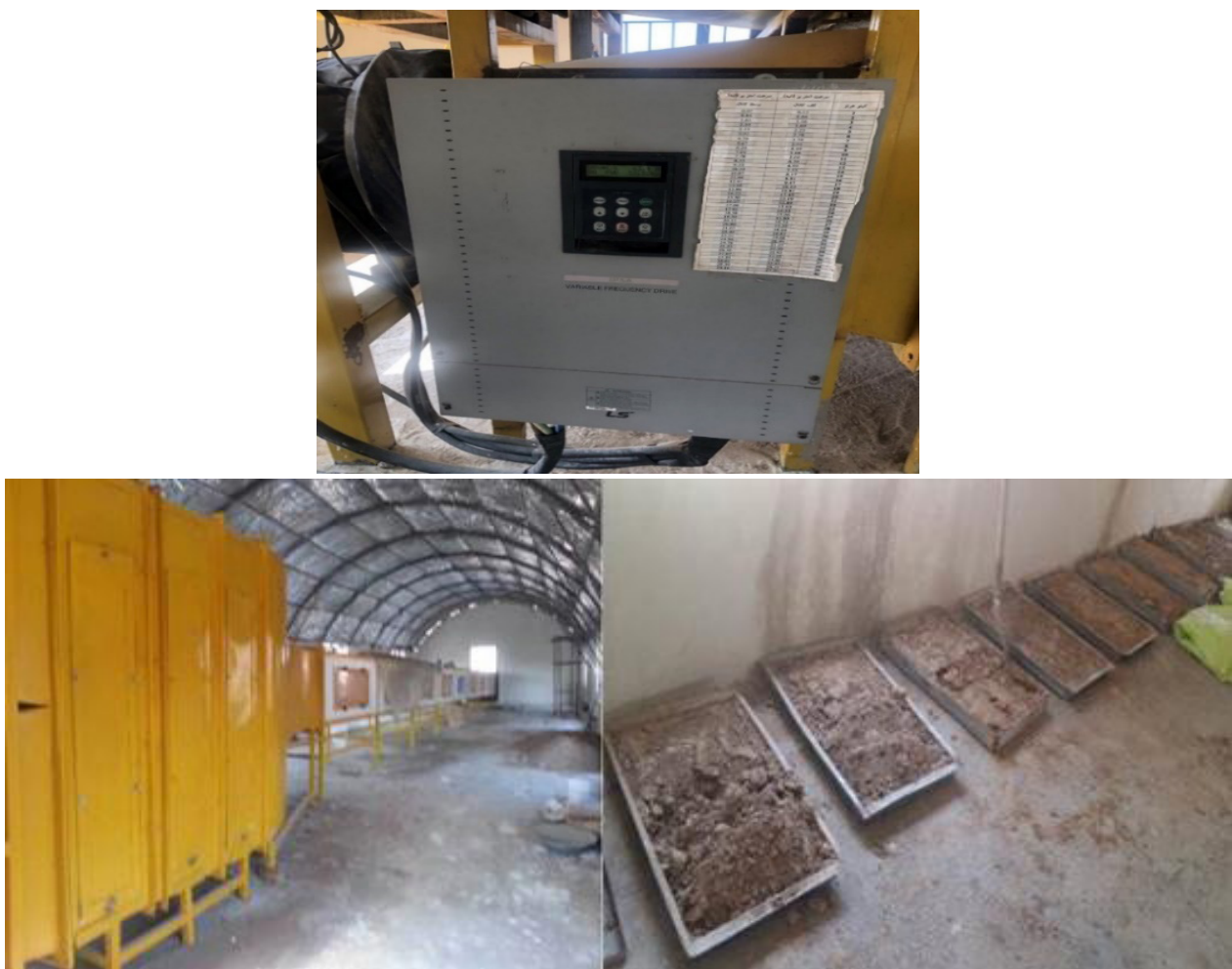
Figure 3) Wind erosion laboratory, constant wind tunnel (left) and settings section (top), and sample under test (right).
