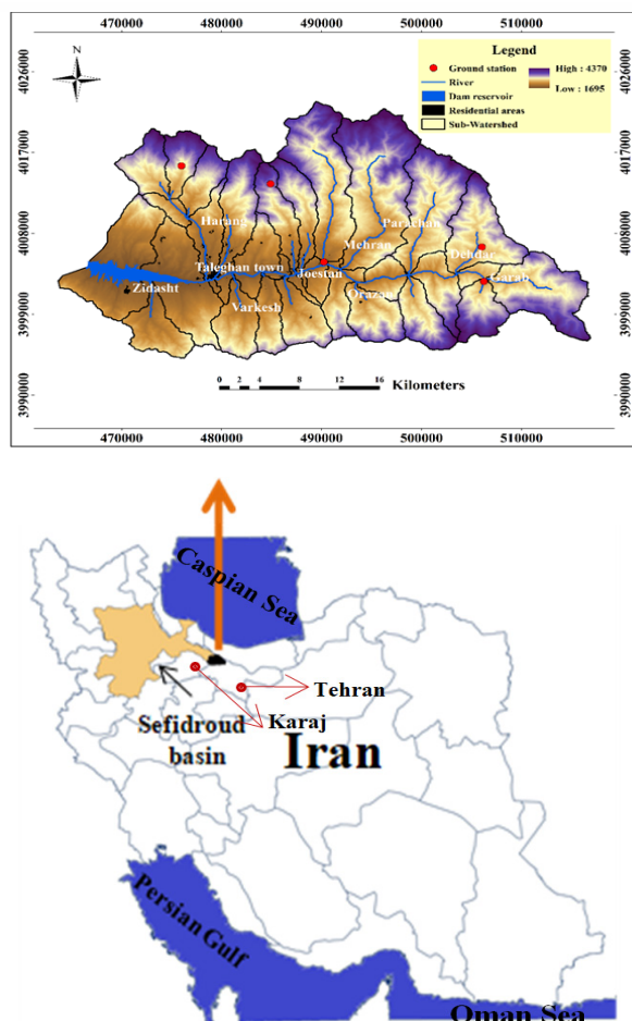
Figure 3) The delineation of the Taleghan Dam Watershed into SWAT with 31 sub-watersheds, gauging station, stream networks and the digital elevation model
