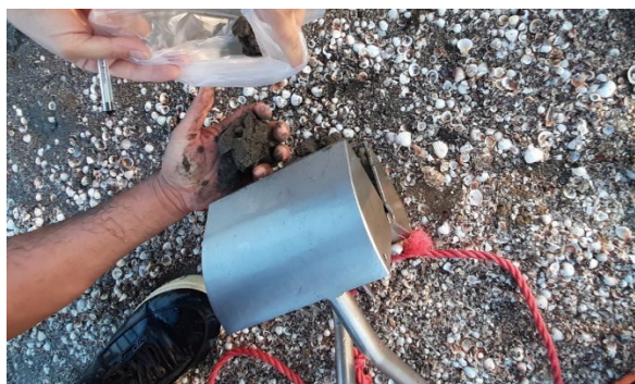
Figure 2) Using Van Veen grab sediment sampler to provide samples from inside each rip channel and control area. Note that during the measurement at sea, it was not possible to provide a suitable photograph for underwater sampling. The provided photo only shows how to work with the Van Veen grab on the beach.
