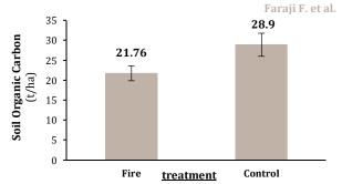
**Diagram 2)** Comparison of the mean soil carbon mass in fire and control sites by Tukey's comparison test
