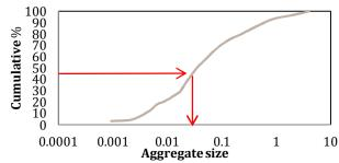
**Diagram 3)** Wet aggregate size distribution curve for studied clayey soil
