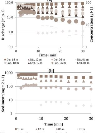
**Diagram 1)** The variations of discharge, sediment concentration (a) and sediment load (b) by time for simulated 1, 6, 12 and 18m slope lengths
