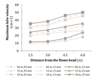
**Diagram 2)** Maximum flow velocity over flume length in three times
