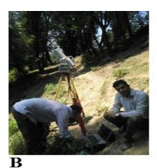
Figure 2 Schematic picture (A) pick up point cloud data by TLS (B) laser scanner field set up
