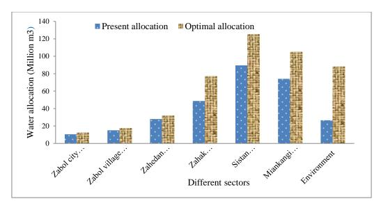
**Figure 3** The present and optimal annual water allocation of the Chahnimeh reservoirs for domestic, agriculture and environment sectors
