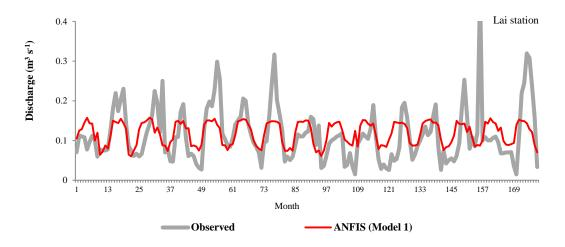
**Figure 4** The simulated hydrographs of the ANFIS models in the training period in comparison with the observed data
