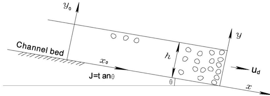
Fig. 1 Definition sketch of the moving coordinates.
