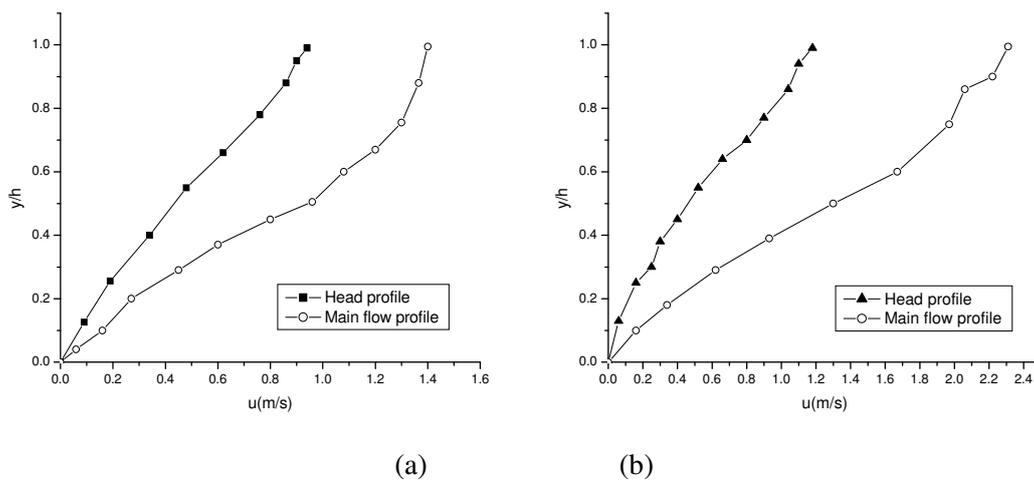
Fig. 5 Velocity profiles of particles in the head and the main flow measured in the two-phase debris flow experiments: (a)  $D_{50} = 20$  mm,  $J = 0.278, h = 0.09$  m and propagation velocity of the debris flow wave is 0.6 m/s. (b)  $D_{50} = 20$  mm,  $J = 0.278, h = 0.12$  m and the propagation velocity of the debris flow wave is 0.7 m/s.
