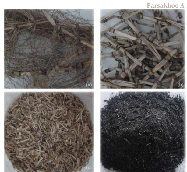
Figure 3) Horsetail ash production; a) air-dried horsetails, b) separated nodes, c) node chips, d) ash
