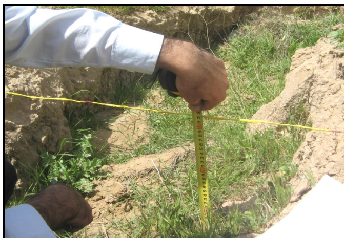
Figure 3 Measurement of gully depth using a thread scaled with 25 cm intervals
