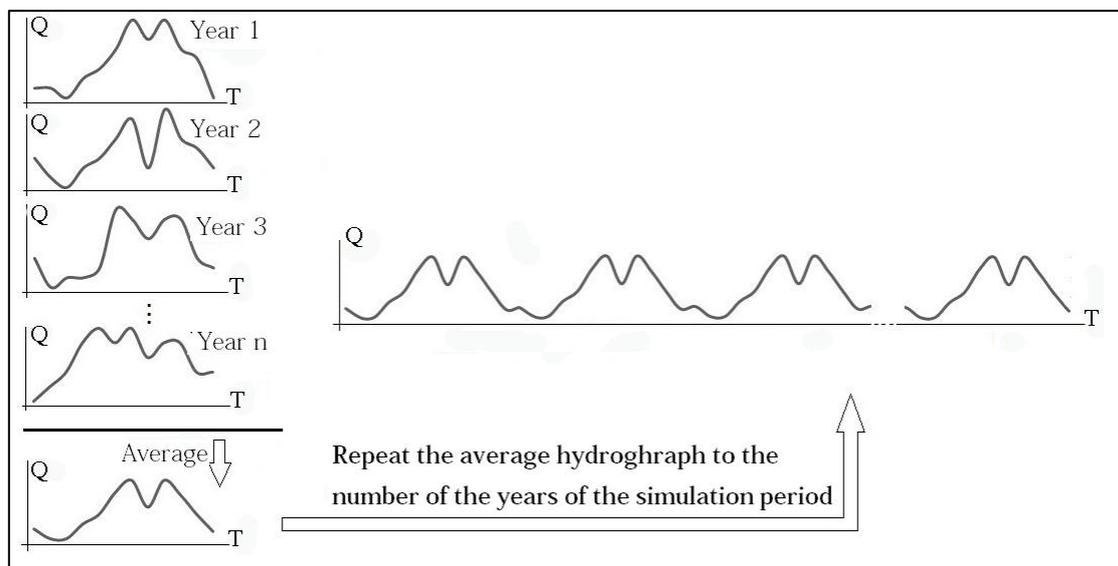
**Figure 3** Calculation processes of the AMH parameter
