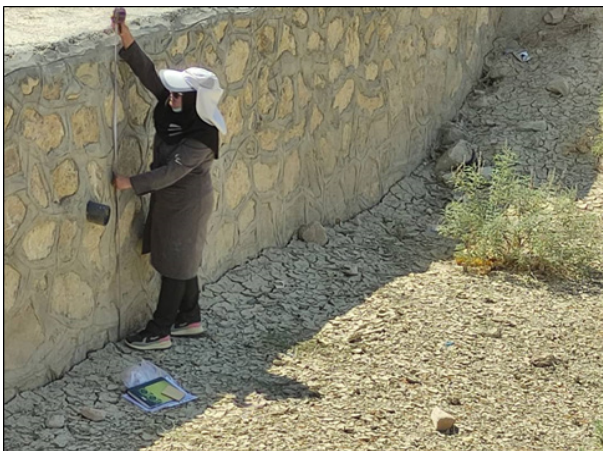
Figure 3) Measurement of the sediment deposited depth.
