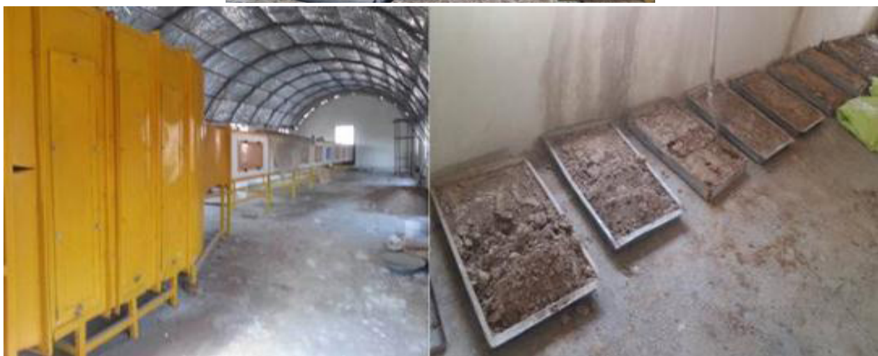
Figure 3) Wind erosion laboratory, constant wind tunnel (left) and settings section (top), and sample under test (right).
