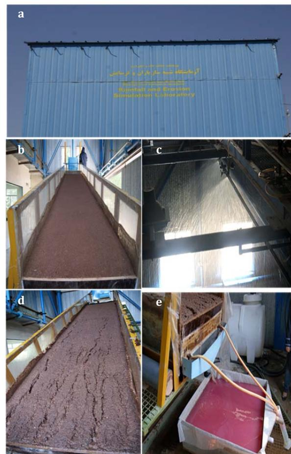
**Figure 1)** Erosion and rainfall simulation laboratory (a), Tilting Flume and inflow tank (b), Nozzle (c), Eroded soil after treatment (d), and Runoff tank (e)
